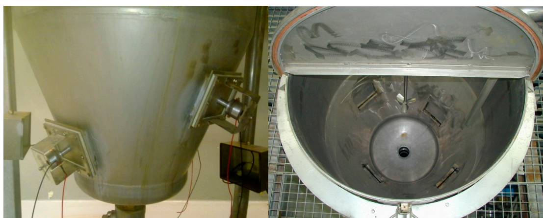
Figure 4. External and internal view of an industrial batch US reactor (300 L) (with kind permission from Martin Bauer, Italy).
