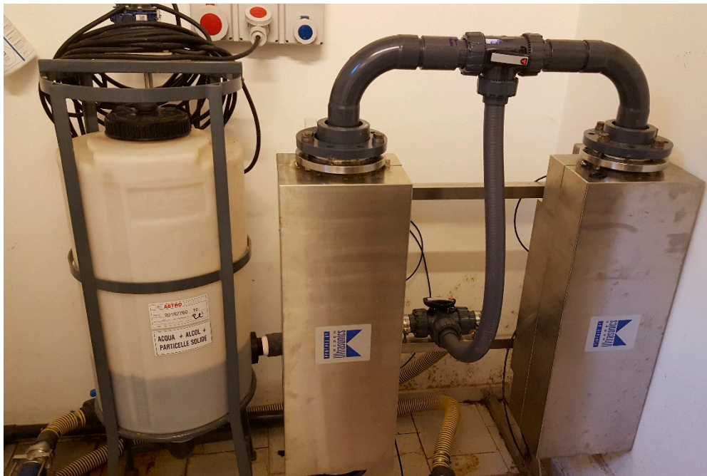
Figure 5. Double-unit, high-power sonochemical reactor (25 kHz and multi-frequency 80–120 kHz) ('green technologies development platform', Dipartimento di Scienza e Tecnologia del Farmaco (DSTF), University of Turin, Turin, Italy).
