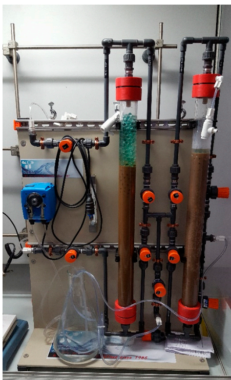
Figure 8. Skid Tecnoimpianti Srl for resin separation ('green technologies development platform', DSTF, University of Turin, Turin, Italy).
