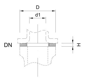
Type CGP...flat gasket for repeated opening and closing for glass connection
