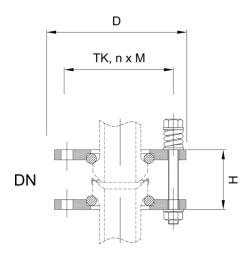
Type CS...-K flange coupling, for glass-glass connection, stainless steel
