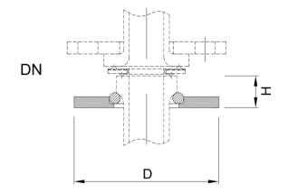
Type CASU...-K adaptor coupling for glass-undrilled connection, stainless steel
