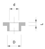
Type CRS...reducing sleeve, for centering M6 or M8 bolts in EN/ANSI flanges.
