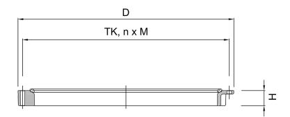
Type CFC...clamp ring for glass connection, die-cast metal.
