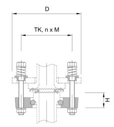
Type CAPG...-K-L... adaptor coupling for glass-enamel flange, plastic
