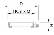
Type CFK... die-cast metal compact backing flange
