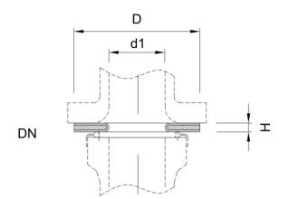
Type CGS...steel core sealing gasket for glass connection
