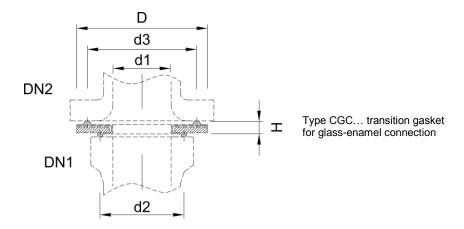
Transition gaskets are clamped and can be connected to flanges in accordance with EN 1092-1 (all nominal diameters) and ANSI 150 (apart from nominal diameters of 25). You will find the relevant adaptor coupling for glass flanges in this chapter.
