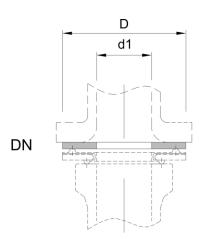
Type CGF...flat sealing gasket for glass connection
