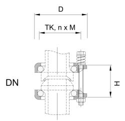
Type CAK...-K compact flange coupling, for glass-glass connection, die-cast metal clamp ring
