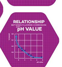
Corrosion progress VL in relation to pH value; in a solution with 19 mmol/I Fluoride at 80 °C.
