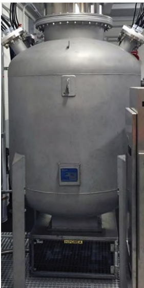
Figure 2: shows one of a large number of a stainless-steel storage tanks lined with Edlon® PTFM (modified PTFE) bonded liner with Pure-Fusion™ Seaming Technology. Edlon designs, fabricates and line all storage tanks for use in Ultra-High Purity applications.
